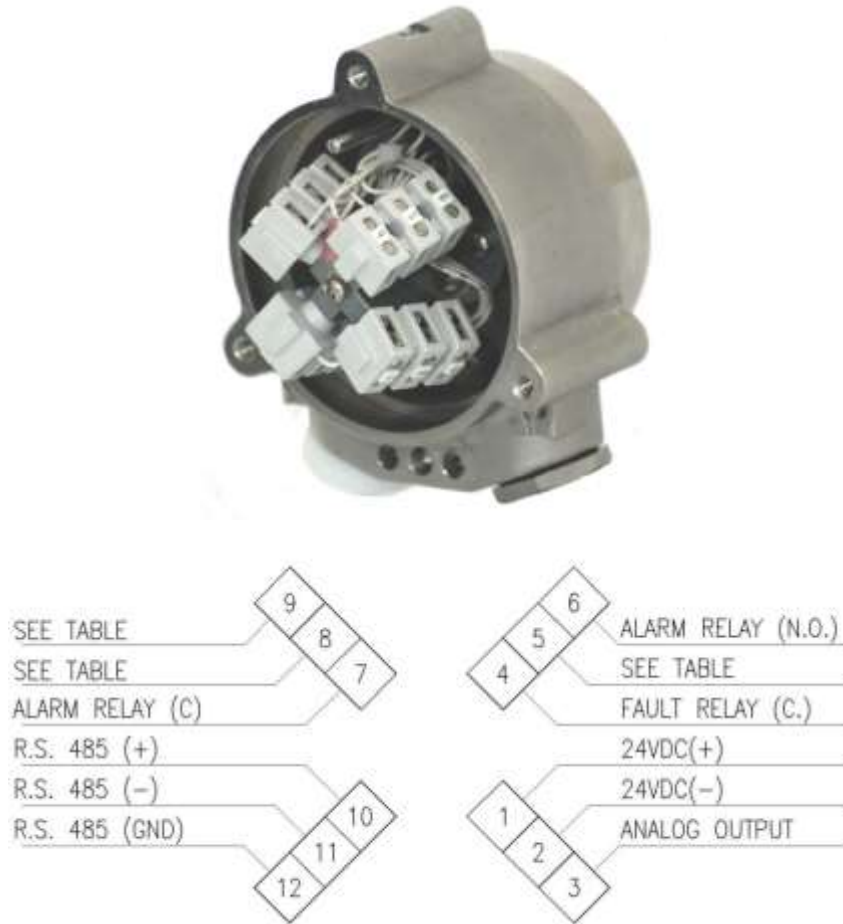
Figure 8: Wiring Terminals
