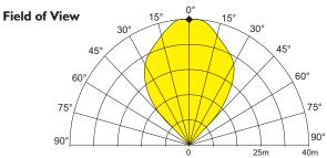
To meet the requirements of EN54:10 clause 5.4, where the ratio of the response points Dmax:Dmin should not exceed 1.41, the horizontal and vertical viewing angles  $\alpha$  max should not exceed  $\pm 30^{\circ}$ .
