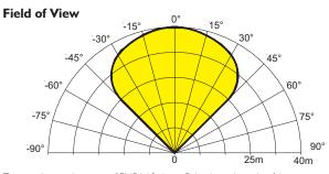
To meet the requirements of EN54:10 clause 5.4, where the ratio of the response points Dmax:Dmin should not exceed 1.41, the horizontal and vertical viewing angles  $\alpha$ max should not exceed  $\pm 30^{\circ}$ .
