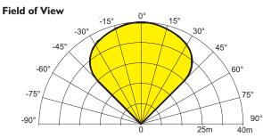
To meet the requirements of EN54:10 clause 5.4, where the ratio of the response points Dmax:Dmin should not exceed 1.41, the horizontal and vertical viewing angles amax should not exceed  $\pm 30^{\circ}$ .
