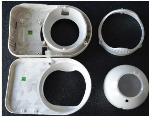
4. Use a screwdriver to open the two halves of the eyeball. You may need to apply a bit of force and choose several locations along both halves to open completely because the eyeball is not designed nor intended for opening.
