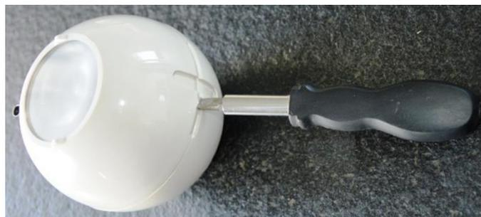
5. When open, remove the top half and note the battery connector.
