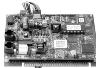
MDACT - Multi-Point Digital Alarm Communicator Transmitter
