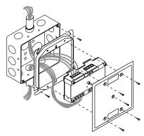
**GSA-MRM1:** mount the UIOxR motherboard inside a suitable Edwards enclosure with screws and washers provided. Plug the module into any available position on the motherboard and secure the module to the motherboard with the captive screws. Wiring connections are made to the terminals on the motherboard (see wiring diagram). UIOxR motherboard terminals are suited for #12 to #18 AWG (2.5 mm2 to 0.75 mm2) wire size.
