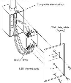
**GSA-MCT2:** mount the UIO motherboard inside a suitable Edwards enclosure with screws and washers provided. Plug the GSA-MCT2 into any available position on the motherboard and secure the module to the motherboard with the captive screws. Wiring connections are made to the terminals on the motherboard (see wiring diagram). UIO motherboard terminals are suited for #12 to #18 AWG (2.5 mm² to 0.75 mm²) wire size.
