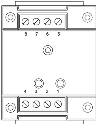
The Signature Series Dual Input Module (model GSA-CT2) is an analog addressable device used to connect one or two Class B, normally open, alarm, supervisory, or monitor type dry contact initiating device circuits (IDCs) to a Signature loop controller. Two device addresses are required.
