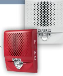
**Genesis strobes** offer 15 to 110 candela output, which is selectable with a conveniently located switch on the side of the device. The current is only 28mA VDC and 36mA VFWR for all light output settings. The candela output setting remains clearly visible even after final installation, yet it stays locked in place to prevent unauthorized tampering. (Data Sheet K85001-0668)
