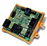
The GSA-REL Releasing Module is an Intelligent addressable device that works with fire suppression systems designed to release extinguishing gas such as Halon. Its primary function is the control of sprinkler pre-action routines and the initiation of suppression system deluge functions. The module is easily configured in the field and offers a wide range of options that
