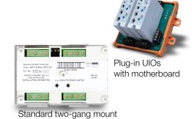
The actual function of each module is determined by its installer-selected personality code. This is downloaded to the module from the device controller during system configuration. Because they are intelligent devices, all decisions are made at the module. This allows lower communication speed but very fast control panel response time and less sensitivity to line noise and loop wiring properties. As a result, twisted or shielded wire is not required.
