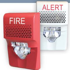
**Genesis strobes** offer 15 to 75 candela output, which is selectable with a conveniently located switch on the side of the device. The current is only 24mA VDC and 32mA VFWR for all light output settings. The candela output setting remains clearly visible even after final installation, yet it stays locked in place to prevent unauthorized tampering. (Data Sheet K85001-0667)
