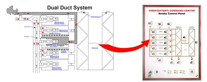
The smoke control system application is conveyed on the BSC Annunciator utilizing illumination, appropriate switch configuration and color to create a visual aid to quickly identify a building's Smoke Control System components.
