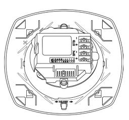
Adjust candela setting by turning dial with screwdriver. Candela selection is displayed on front of unit.
