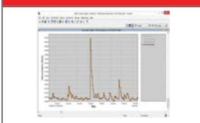
DustTrace is an optional software analytics that can be licensed for the VESDA-E series of aspirating smoke detectors. It provides targeted detection of dust which is present in the sampled air.
