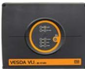
The VESDA VLI is an industry first early warning aspirating smoke detection system, designed to protect industrial applications up to 2,000 m<sup>2</sup> (21,520 ft<sup>2</sup>). The VLI detector combines a patented fail-safe Intelligent Filter with Clean Air Zero and clean-air barrier for optics protection complementing absolute detection and providing longer detection chamber life all enclosed in a robust IP66-rated enclosure.
