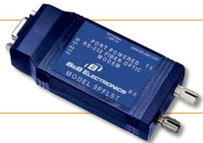
These port-powered fiber optic modem allows two RS-232 serial devices to communicate transparently over longer distances and with greater reliability. The inherent immunity of fiber optic protects data from line surges, spikes and ground loops.
