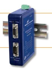
The 2320PDRI is our premium Industrial RS-232 Isolated Repeater. Designed for rugged industrial environments, it is UL listed and certified for use in Class 1 Division 2 locations. Powerful Optical Isolation on both data ports protects your equipment and data from damaging ground loops and surges. Additional isolation on the power supply circuits adds a third degree of protection.
