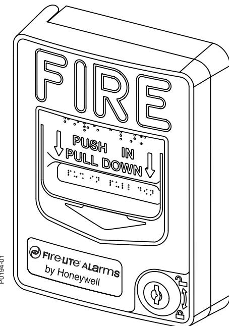
**NOTE:** Closing the door automatically resets the switch to the 'Normal' position.
