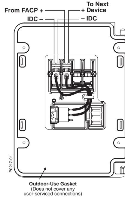
**WARNING!** Do not loop wiring under any terminals. Break wire run to maintain IDC supervision.
