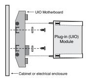
**SIGA-MIO:** mount the UIOxR motherboard inside a suitable EDWARDS enclosure with screws and washers provided. Plug the module into any available position on the motherboard and secure the module to the motherboard with the captive screws. Wiring connections are made to the terminals on the motherboard (see wiring diagram). UIOxR motherboard terminals are suited for #12 to #18 AWG (2.5 mm² to 0.75 mm²) wire size.
