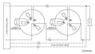
Note: If a remote annunciator is not used, polarity of these terminals may be reversed.
