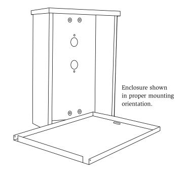
Cut the two sampling tube openings using a  $1^3/8''$  hole saw or hole punch. Drill the remaining six holes (0.17" diameter) using a #21 drill bit. Using the screws provided, secure the enclosure at the four corners.
