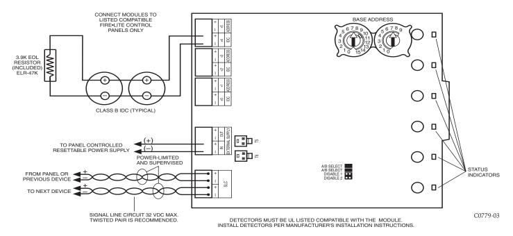
To use a common power supply between multiple MMF-302-6 modules, connect a long power supply jumper from T5 or T6 to T5 or T6 on the adjacent MMF-302-6 module.
