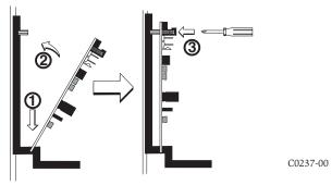
Step 1: Insert the bottom of the MMF-302-6 module down into a rear slot on the chassis.
