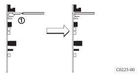
Step 1: Insert the bottom edge of the MMF-302-6 module down into a rear slot of the chassis.
