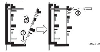
Step 1: Insert the bottom edge of the MMF-302-6 module down into a front slot of the chassis.
