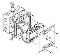
**SIGA-MRM1:** mount the UIOxR motherboard inside a suitable GE Security enclosure with screws and washers provided. Plug the module into any available position on the motherboard and secure the module to the motherboard with the captive screws. Wiring connections are made to the terminals on the motherboard (see wiring diagram). UIOxR motherboard terminals are suited for #12 to #18 AWG (2.5 mm2 to 0.75 mm2) wire size.
