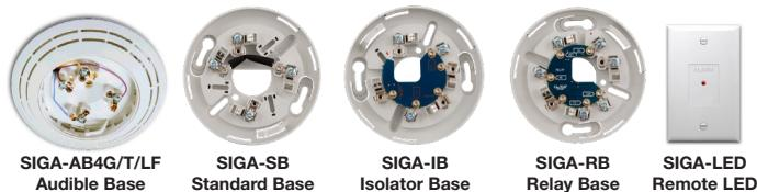
**Remote LED SIGA-LED** - The remote LED connects to the SIGA-SB or SIGA-SB4 Standard Base only. It features a North American size 1-gang plastic faceplate with a white finish and red alarm LED.
