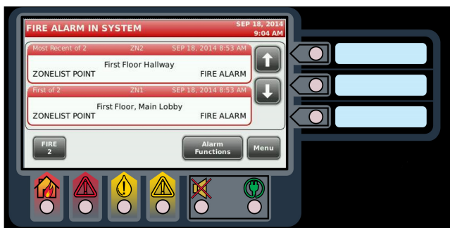
Figure 2: Touchscreen display with LED status indicators
