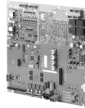
FCI2017-U1 (Periphery board for 504-point Desigo Fire Safety system)
