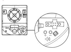
Test points indicated above are used to validate the Notification Appliance Circuit and verify device function.
