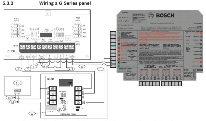
Figure 5.5: Wiring two-wire loops for power supplied by an external auxiliary power supply controlled by a relay and a G Series panel
