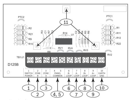
Figure 2.1: D125B Powered loop interface
