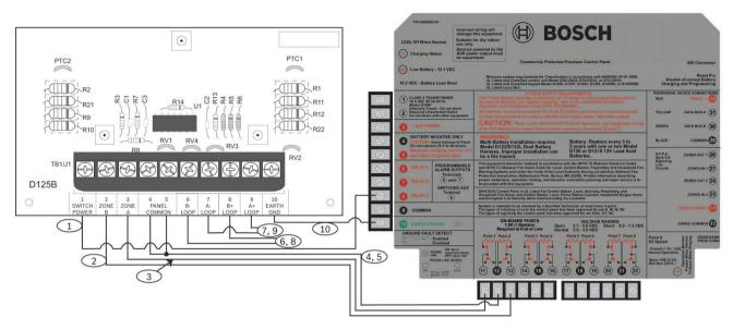
Figure 5.3: Wiring two-wire loops powered by a G Series panel
