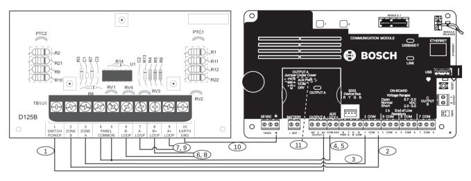
Figure 5.2: Wiring two-wire loops powered by a B Series panel
