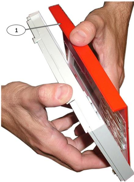
**Figure 6: Removing the Red Cover**
