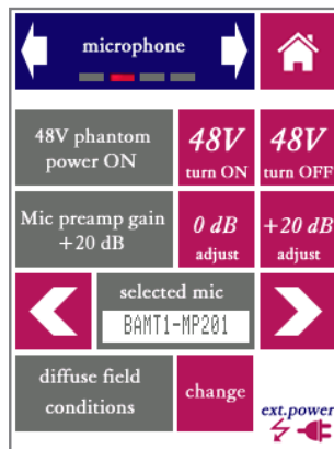
The microphone and preamp settings: turning phantom power on/off, selecting the preamp gain (measuring range), selecting the microphone type, and selecting free field or diffuse field measurements.
