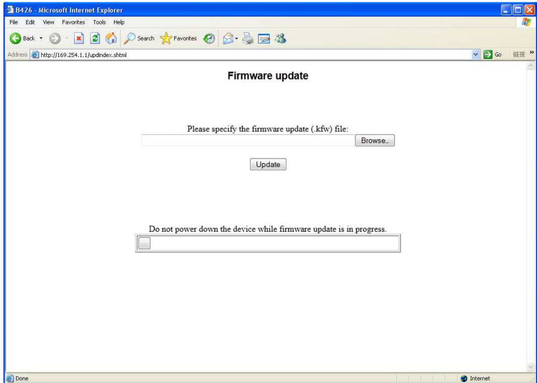
Figure 5.10: Firmware upgrade specify upgrade file
