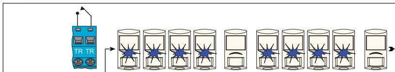
**Self-tests every 8 h. Self-test and remote self-test failure: 4 blue flashes**
