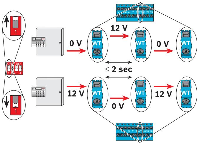
Trouble Memory: Pulse WT input to recall last trouble condition from memory. Pulse WT input again to clear memory. When memory is recalled, it automatically clears after 12 h.
