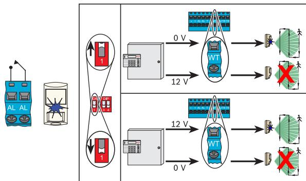
**Remote Self-Test:** Remote Self-test automatically occurs when walk test changes from disabled to enabled (change in terminal voltage).
