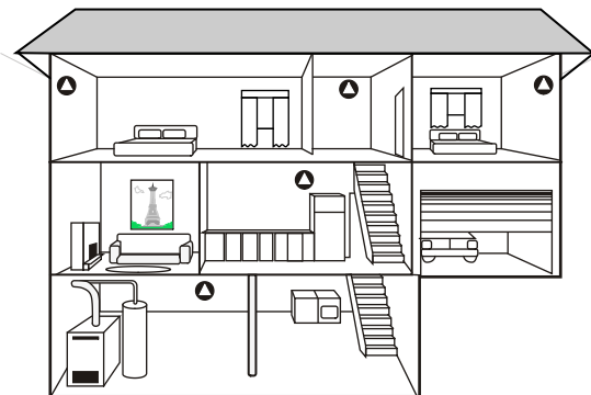
Figure 2: Recommended CO detector locations
