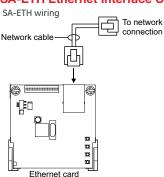
The SA-ETH card provides a standard 10/100 Base T Ethernet network connection for connecting to an intranet, a local network, or the Internet. The card can be used to download configuration programming from the VS-CU to the panel over the network.
