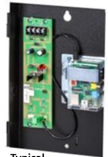
Typical mounting set-up of a SNU module
