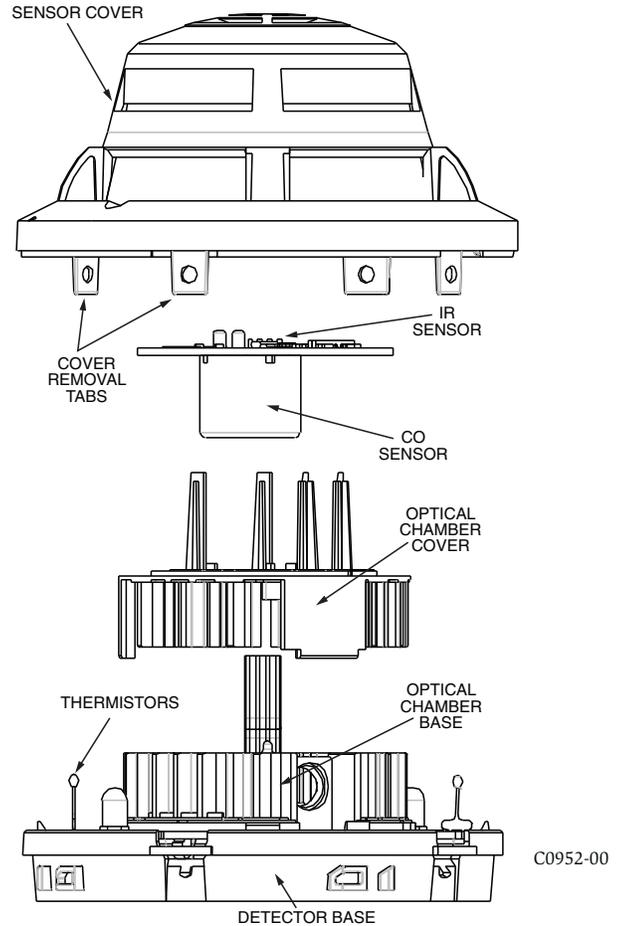
7. Re-install the sensor cover. Use the cover removal tabs, LEDs and thermistors to align the cover with the sensor. Snap the cover into place.
