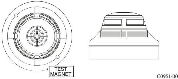
For MIX-COSAP, smoke entry testing should be performed immediately following the magnet test. Magnet test initiates an approximately 10 minute period when the detector's signal processing software routines are not active. Failure to first perform the magnet test will introduce a time delay before the detector alarms.
