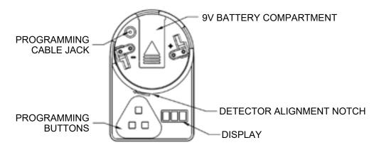
NOTE: Prior to programming, ensure battery is connected.
