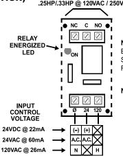
NOTE: INPUT POWER SUPPLY SHOULD BE UL LISTED FOR FIRE PROTECTION SIGNALING SYSTEMS WHEN USED IN FIRE ALARM APPLICATIONS
