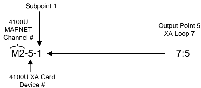
Figure 15. Mapping XALIC Point Names to XA Loop Devices (4100U Shown)
