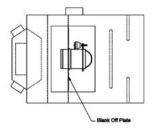
Titus® HD,TDH,TDL,TSH, LD, HS Series Replace all mechanical regulators with combination of flanged retrofit assembly(ies) and blank off plate(s) through bottom access panel. One actuator per valve, field or factory mounts on valve body. Flow controller panel is mounted in the field on outside of HD air terminal casing.
