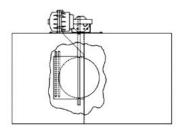
Barber-Colman® HS and HD Series Replace mechanical regulator(s) with panel mounted single or dual round or oval retrofit valves. Retrofit is achieved through a side access panel. One actuator and flow controller are mounted on outside of the HS or HD side access panel in the field.
