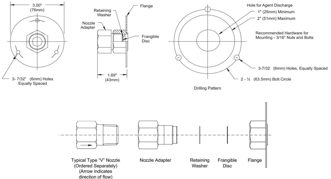
**Note:** Shipped assembled without the Type "V" Nozzle.
