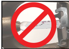
INCORRECT (bulb cracked, fluid missing)
