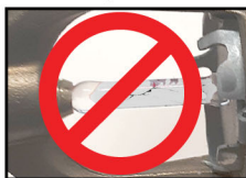
INCORRECT (bulb cracked, fluid missing)
