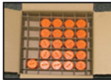
CORRECT (Protective caps in place)
