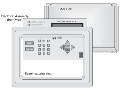
Assembled annunciator also includes mounting wires, 2 set screws.
