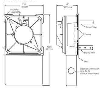
**Note:** The AD-HR air duct housing is used with HFP-11 detectors on the FireFinder XLS control panel when a relay is required in the housing. If no relay is required, use the AD-11P housing.
