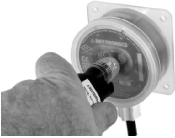
Figure 2—Testing a PM-5MP+ Using a PSS-ML Test Lamp
