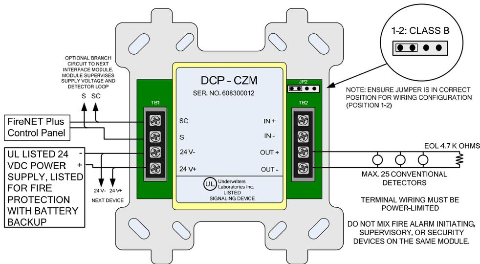
Figure 5.14.1 CZM Conventional Zone Module, Style B
