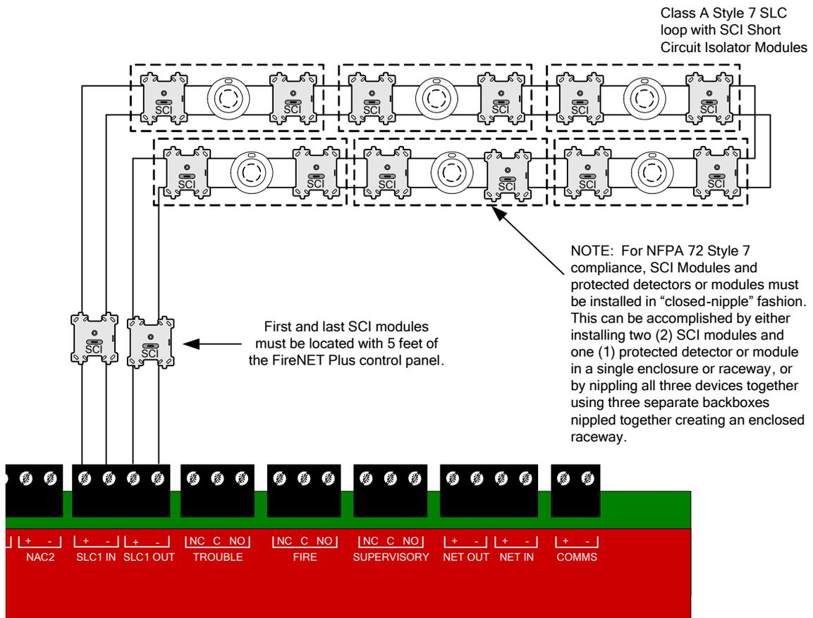
Figure 5.15.2 Style 7 SLC Circuit Example
