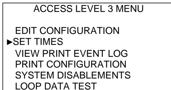
The SET TIMES menu option allows the installer to set the smoke detector calibration time, the day / night sensitivity times, and the Sounder Time-Out for the panel.
