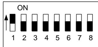
This switch setting shows address number one. Switch position up selects the binary digit, so a switch with 1,2 and 3 up would represent address number 7.
