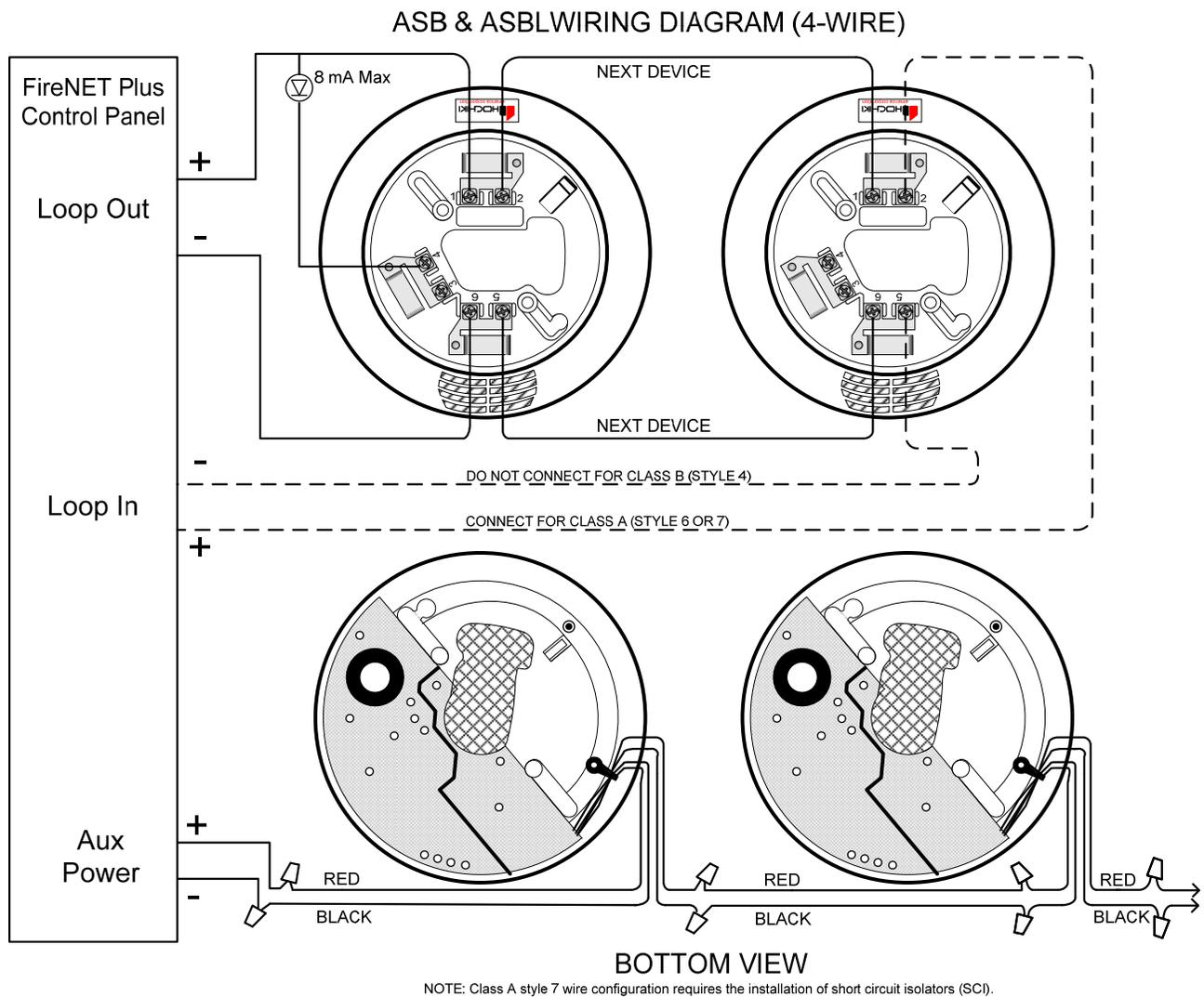
**Figure 5.16 ASB & ASBL Analog Sounder Base Connections**
