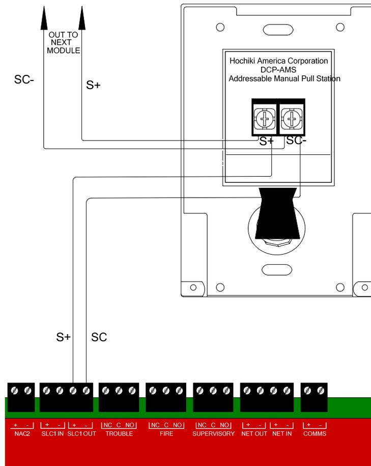
Figure 5.17.1 AMS Addressable Manual Pull Station Wiring Detail
