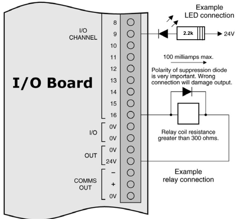
**NOTE:** Outputs on the I/O board are not supervised. These outputs are not for primary notification of fire conditions (i.e. not for use as NAC circuits). These outputs are for secondary use only. All primary notification output devices must be connected to applicable NAC circuits on the FireNET panel. See Section 3.4, Appendix A, and B for details on NAC circuits and compatible NAC devices.
