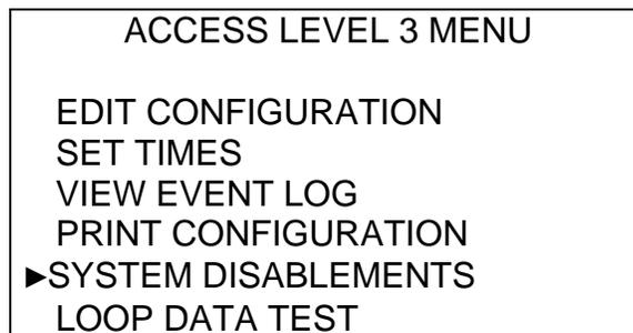
The System Disablements menu option allows the installer to temporarily disable the panel buzzer, ground fault detection, and set the buzzer silence access level. The panel buzzer and ground fault detection are enabled in the panel's default condition. The buzzer silence access level is set to 2 by default.
