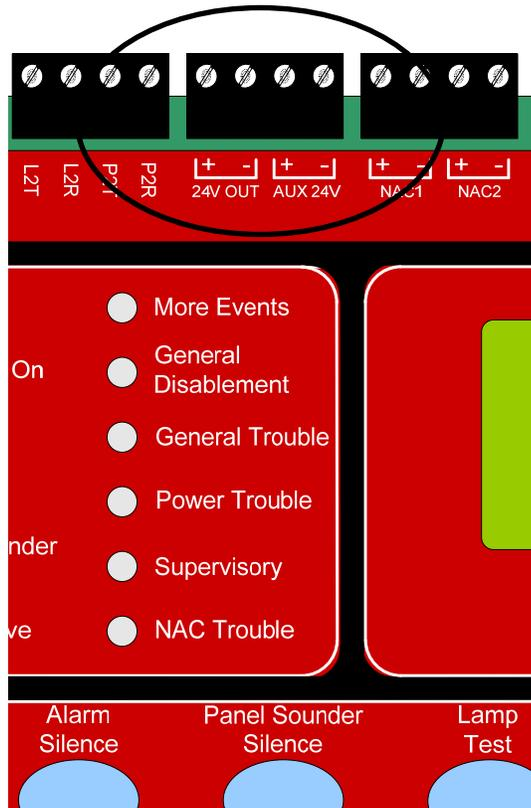
Figure 3.2 Auxiliary Power Connection Detail
