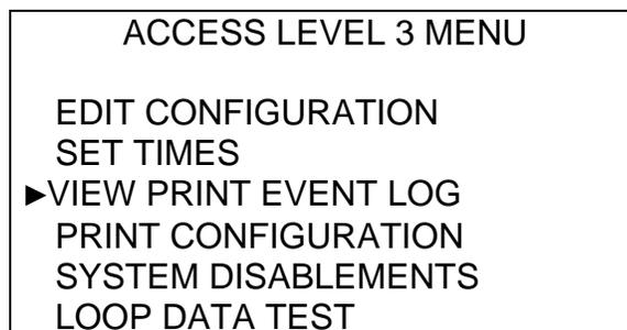
The View Print Event Log menu command allows the user to view the system's 500-event memory log. Any condition outside of normal panel operation generates an entry into the
