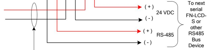
To AUX 24VDC of control panel or to UL 864/1481 listed AUX 24VDC Power Supply
