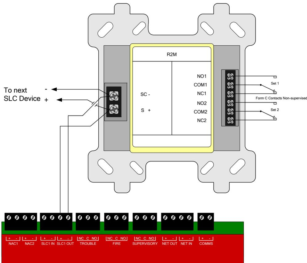
Figure 5.10.1 R2M Dual Relay Module Wiring Detail
