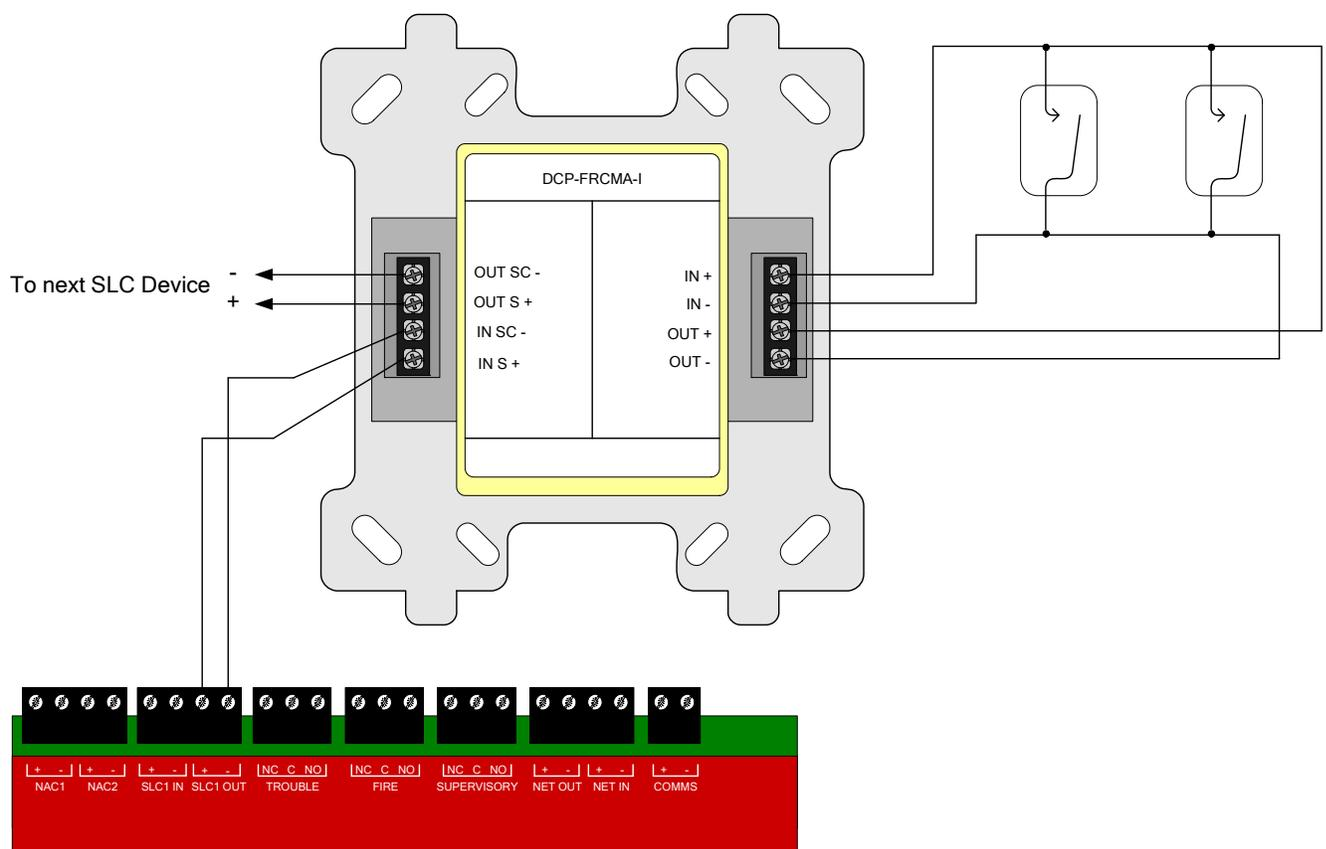
Figure 5.9.1 FRCMA-I Input Module Class A Detail
