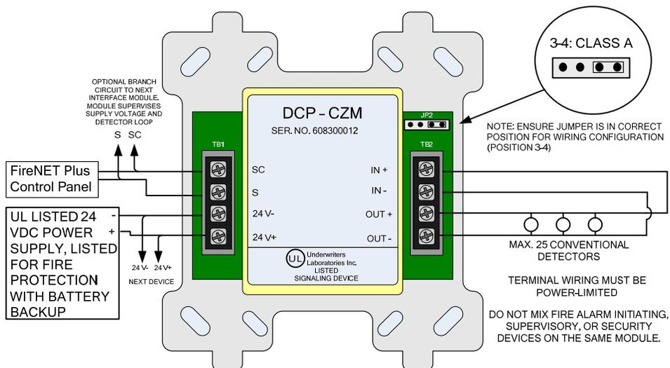
Figure 5.14.2 CZM Conventional Zone Module, Style D
