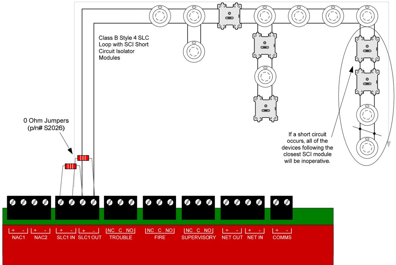
Figure 5.15.3 Class B Operation of the SCI Module
