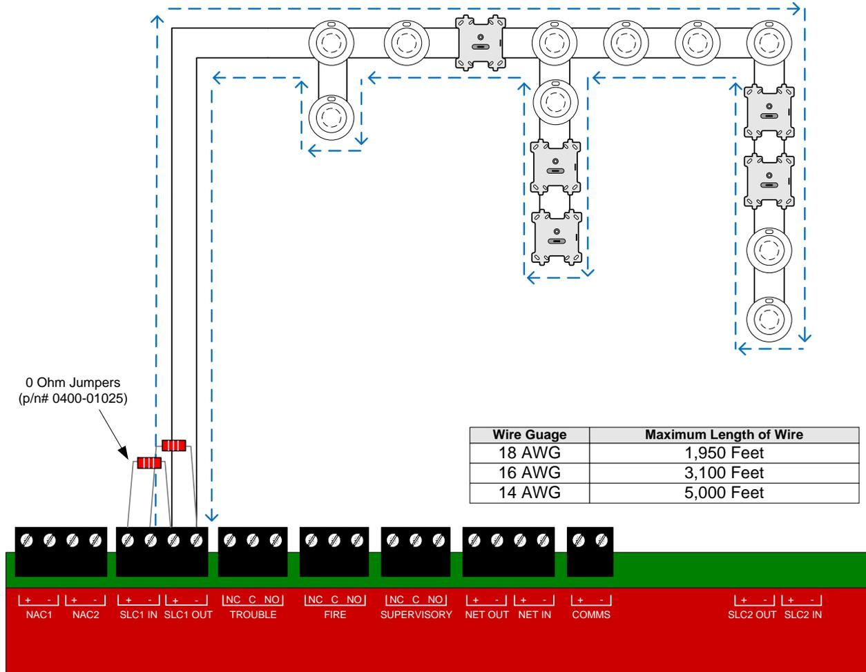
Figure 5.3.2 Maximum Wiring Length for a Class B SLC with T-Taps
