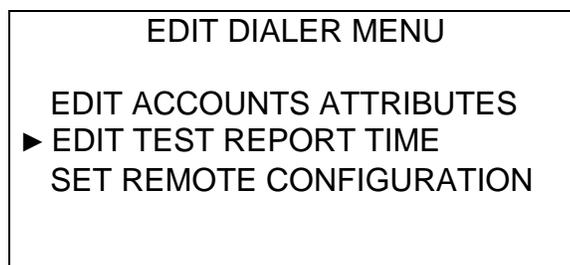
Use the up or down arrow key to select the test report time. The test report will be sent every 24 hours at the time selected. Press the Enter button when the desired time is displayed.
