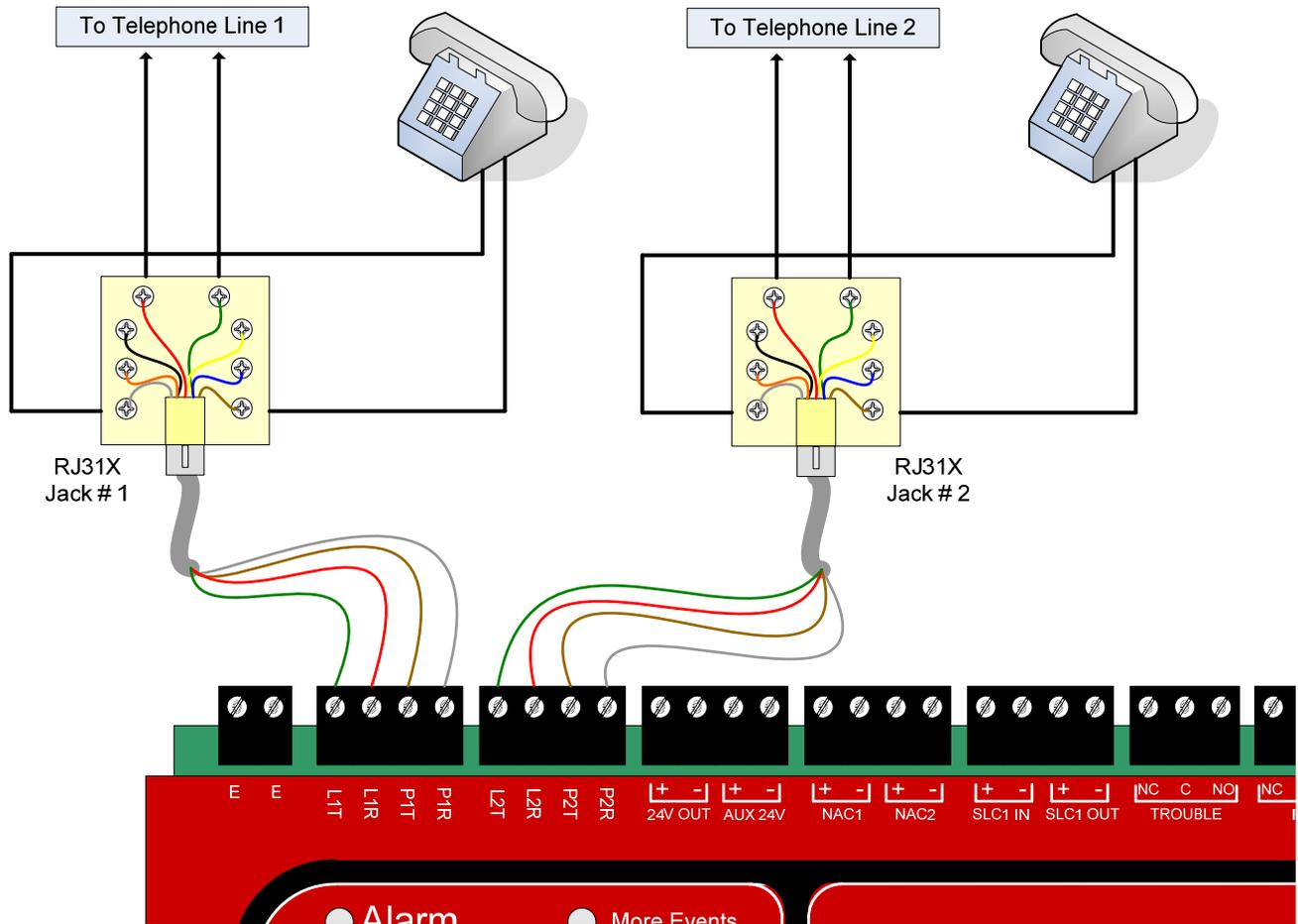
Figure 3.5 – Telephone Line Connections to the FireNET Plus
