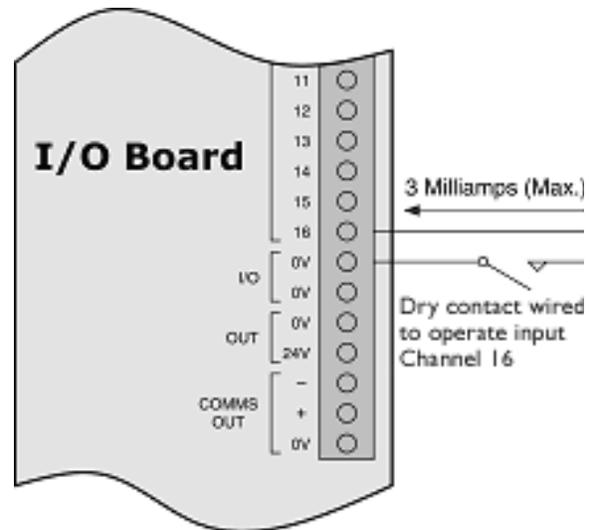
**NOTE:** Inputs on the I/O board are not supervised. These inputs are not for primary initiating or detection of fire or life safety conditions. These inputs are programmable for secondary use only, and not used for signaling Fire, Supervisory, or Trouble conditions. All primary initiating or detection inputs must be connected to applicable SLC devices listed for fire. See Section 5 of this manual for SLC devices.
