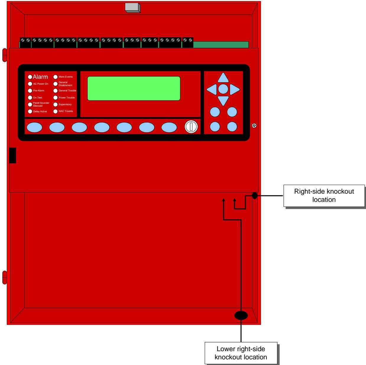
**Figure 2.5.1 – Suggested Routing of AC Power**
