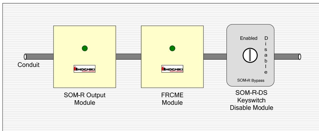
2. The SOM-R must be addressed using the TCH-B100 programmer. Connect the SOM-R to the FireNET Plus SLC as shown in Figure 5.13.1. Refer to the installation instructions (Part # 1700-11320, Rev. 05/10) included with the SOM-R for additional wiring and installation instructions.
