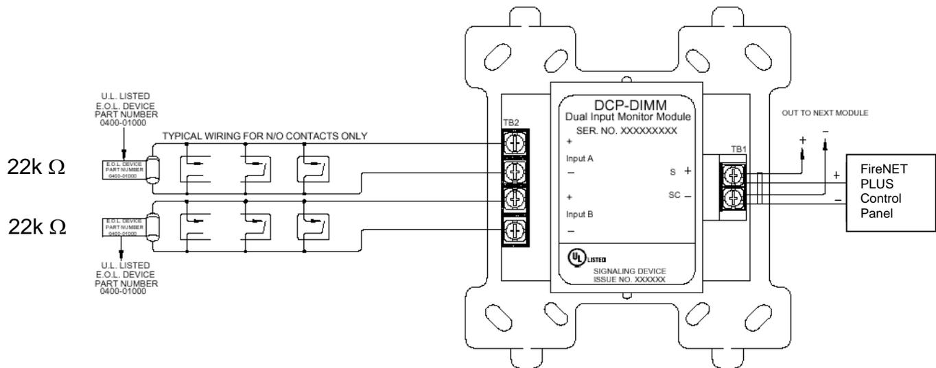
Figure 5.15 DIMM Dual Input Monitor Module Connections
