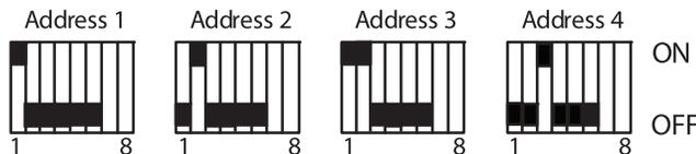
Figure 3. Set the RS-485 address
