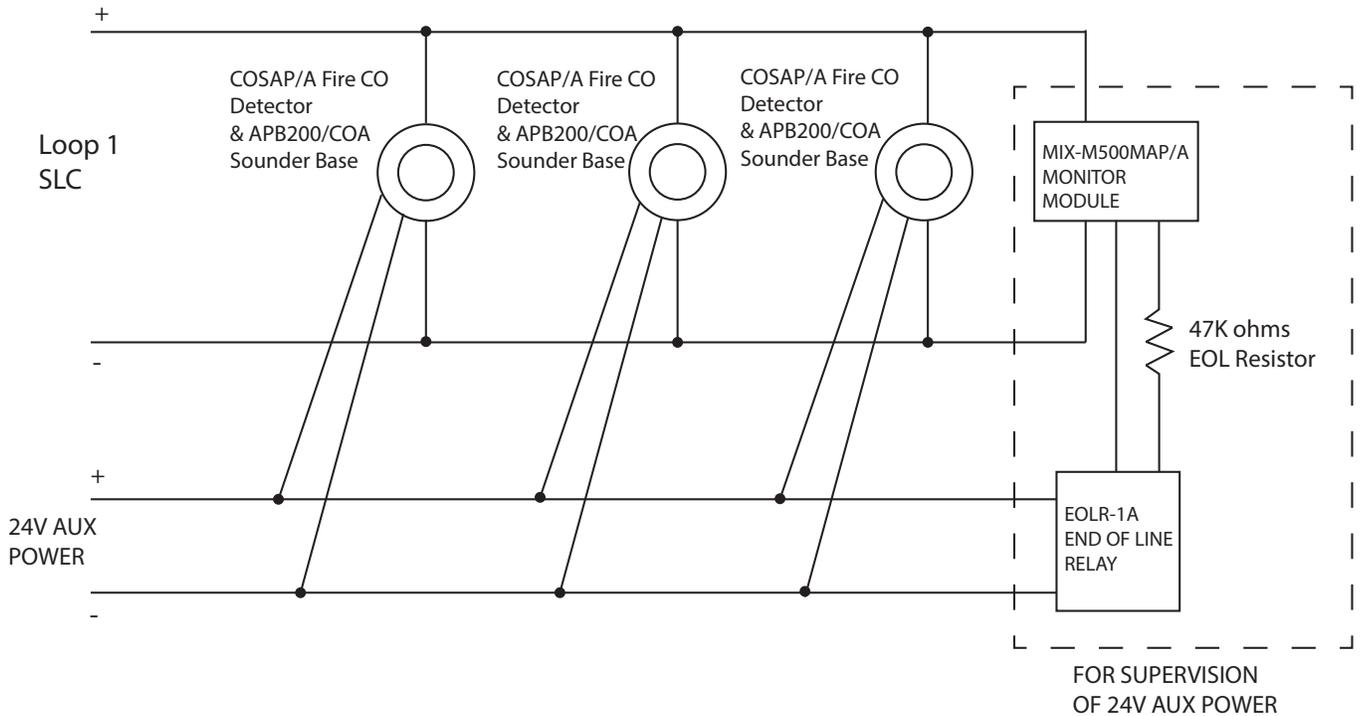
The monitor module (shown in the diagram above) should be set up in the configurator to report as a trouble input with the message tag "Sounder Base Fault".
