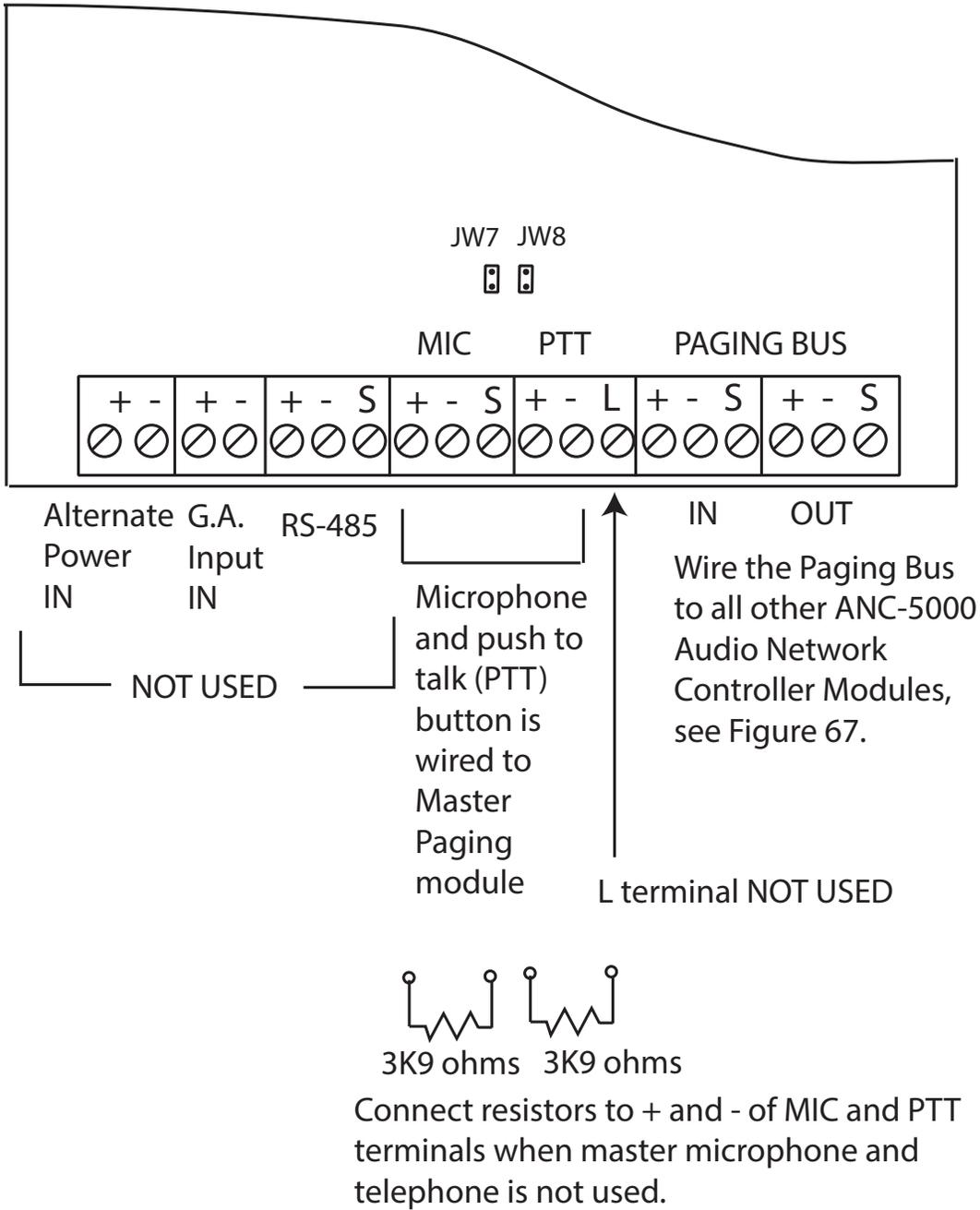
Figure 69: Audio Paging Bus Wiring
