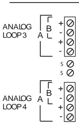
This board is mounted over the ALCN-792MISO loop adder module to provide an addition two loops, for a total of four loops.
