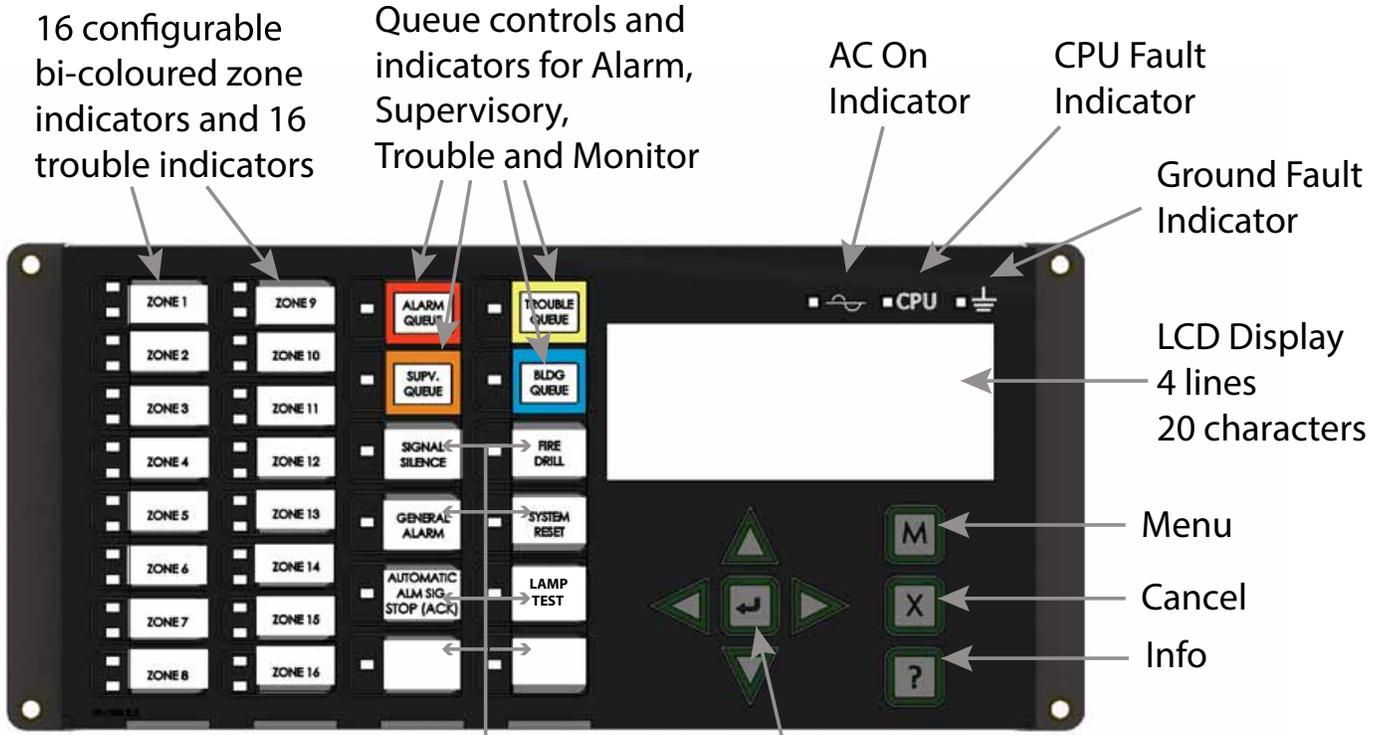
Control and Indicators for Signal Silence, General Alarm, General Alarm Cancel (Automatic Alm Sig Stop (ACK)), Fire Drill, System Reset, Lamp Test (Visual Indicator Test) and Spare programmable Buttons
