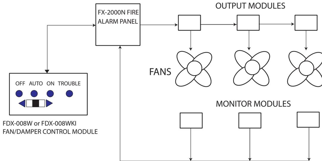
Before mounting the FDX-008WKI module, if a keyswitch is to be connected, wire the keyswitch to terminals at TS1 as shown in Figure 19 below. Mount the FDX-008W and FDX-008WKI Fan Damper Control Display modules in any position on the front part of the FX-2000N chassis and backbox.
