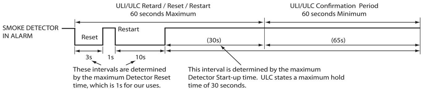
A Manual Station, or other contact-closure device, would remain shorted and be detected during the very short Zone Power burst within the first three seconds. A Smoke Detector will have been reset, and will require some minimum time to power-up, thus the Verification cycle will be entered.
