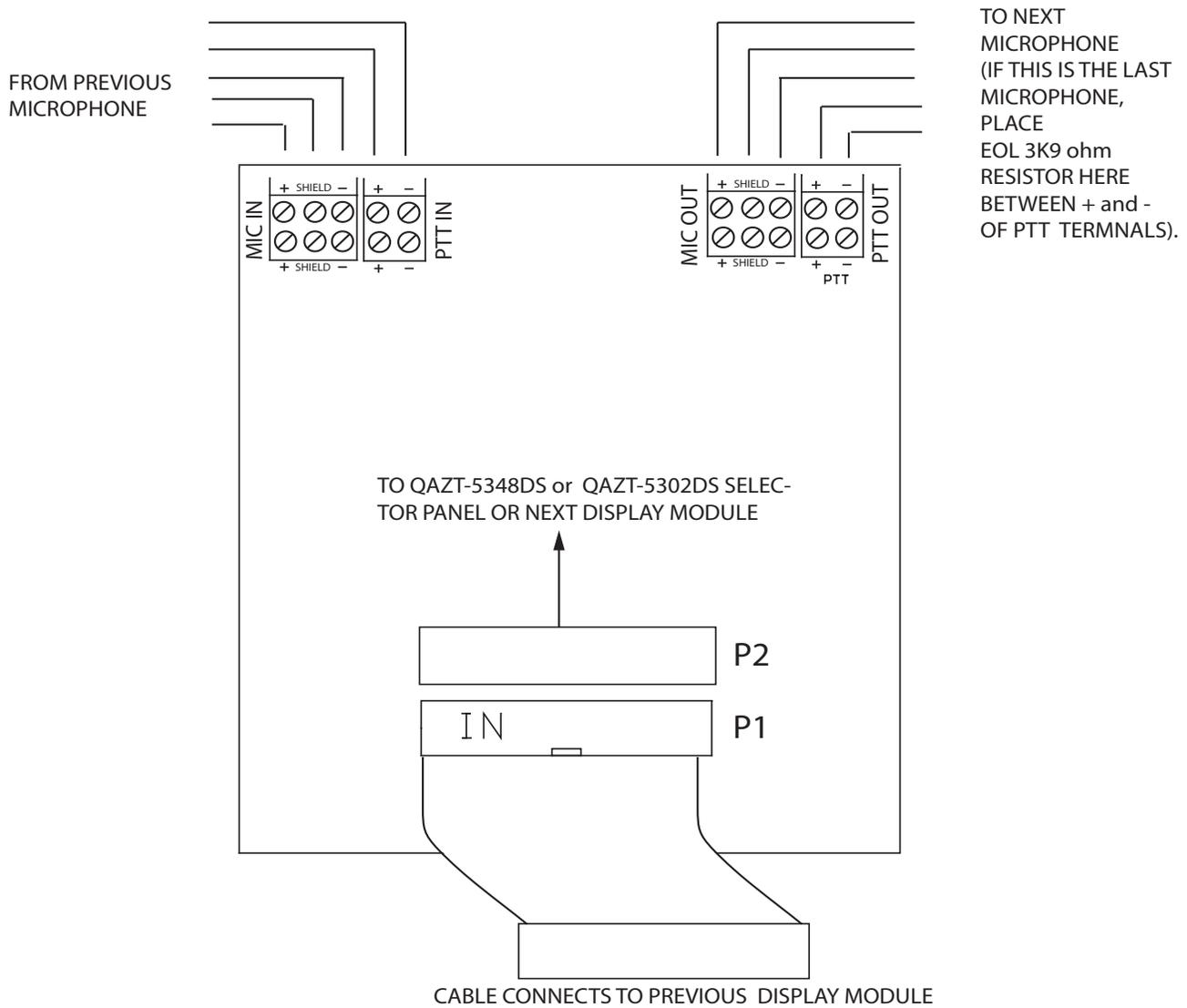
The interface wiring between the QMP-5101N and ANC-5000 is as follows:
