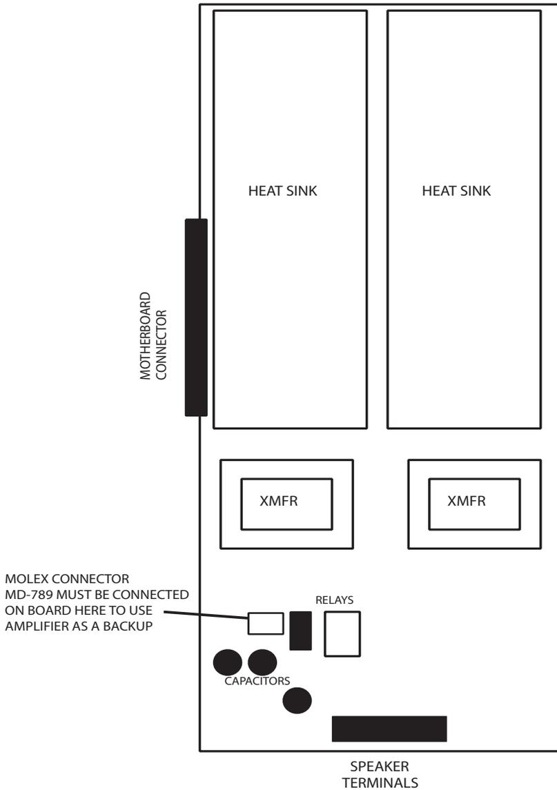
Any amplifier may be designated as the backup amplifier and this backup amplifier must have the MD-789 molex connector placed in the bottom left-hand corner of the board as shown in the adjacent figure. The QAA-5160-70/25 as backup amplifier is inserted into the motherboard. No connections are made to the backup amplifier's terminals except for end-of-line resistors which are to be placed directly on the terminals in the audio cabinet.
