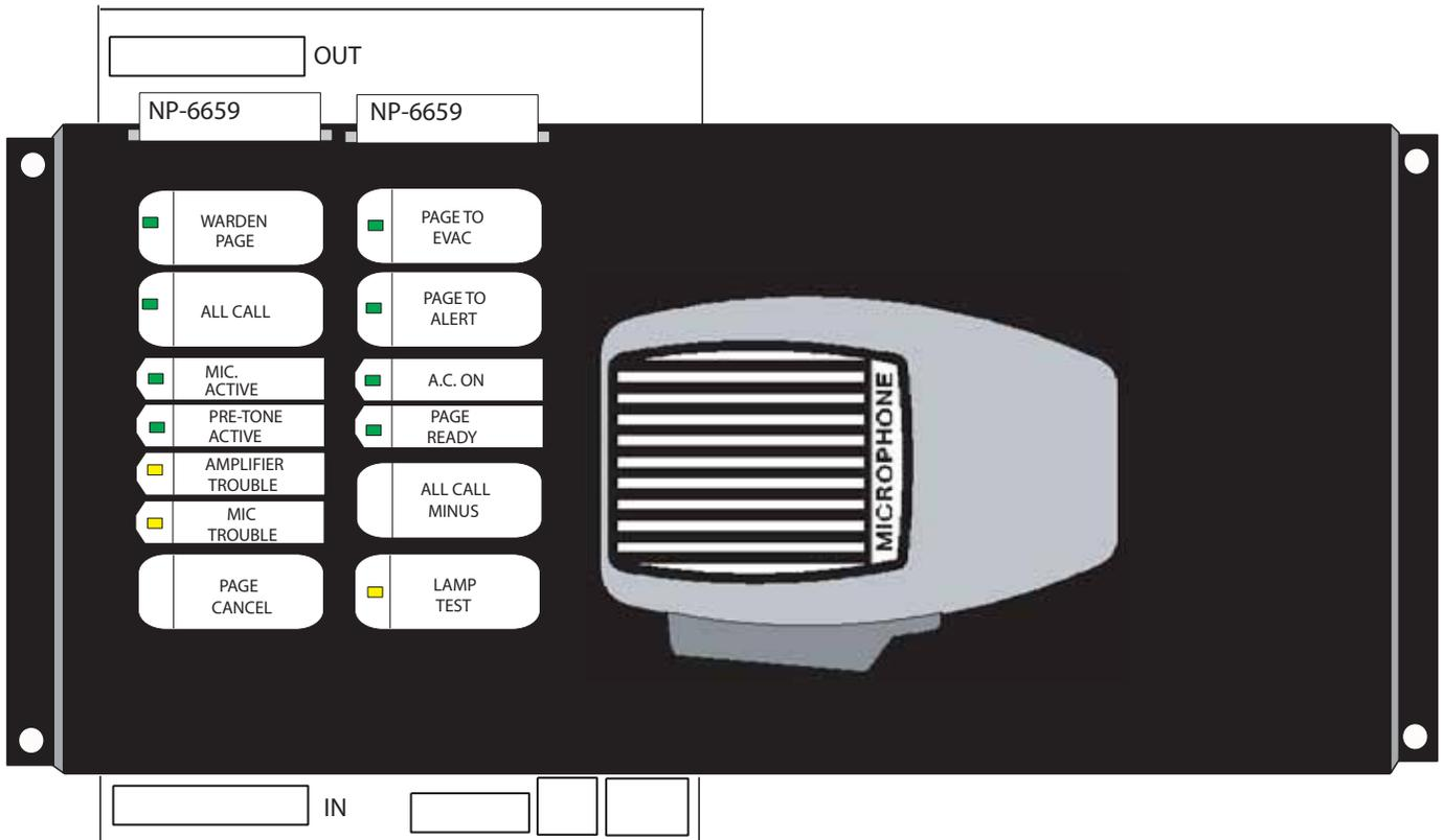
Connect ribbon cable from P1 (IN) to previous display module. Connect P2 (OUT) to the QAZT-5348DS or QAZT-5302DS Zoned Selector Panel or next display module. Wire the positive and negative terminals and the microphone MIC positive, negative and shield to the ANC-5000 Audio Network Controller Module corresponding terminals.
