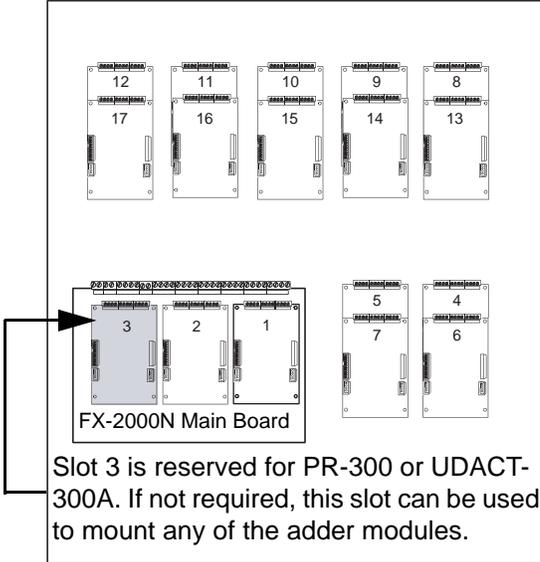
The recommended mounting position is 2 for the FNC-2000. The FOM-2000-UM board, if used, is mounted over the FNC-2000 board.
