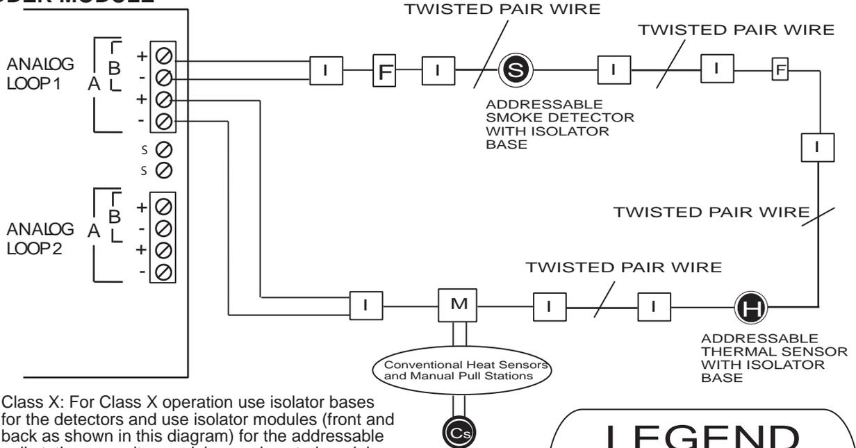
Class X: For Class X operation use isolator bases for the detectors and use isolator modules (front and back as shown in this diagram) for the addressable pull stations, monitor modules, and control modules.
