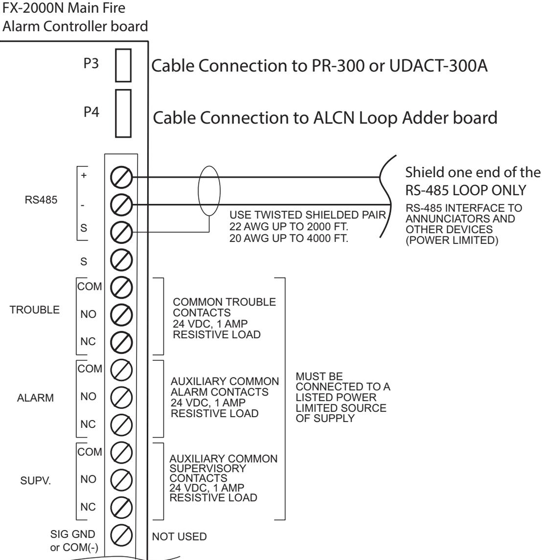
Figure 28: Main Fire Alarm Control board Field Terminal Connections (continued)
