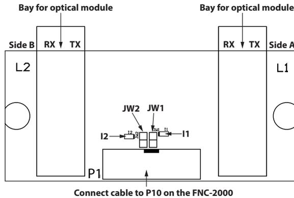
One of these modules is required at each panel where fiber optics will be used between them. The FOM-2000-UM will be mounted over the FNC-2000 Network board (over the field wiring terminals) with two #6 Phillips screws and two Hex spacers.
