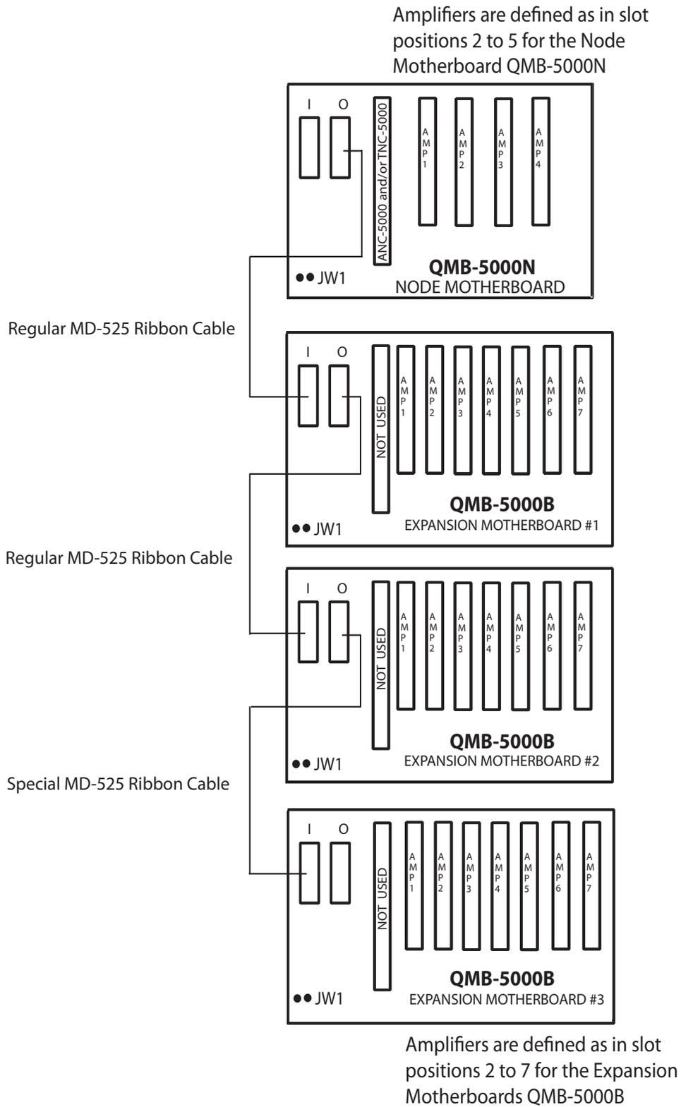
**Note:** Jumper JW1 (located in the bottom left-hand corner of the backplane) is installed for expansion cabinets #1 to 3.
