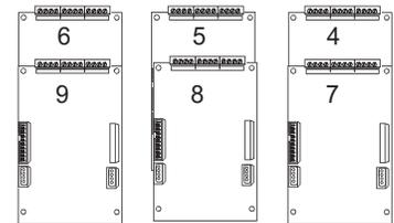
Slot is reserved for FNC-2000. If not required, this slot can be used to mount any of the adder modules.
