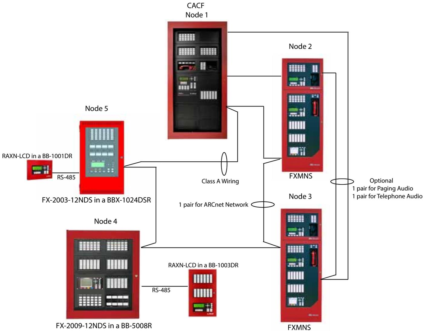
NOTE: Wiring for ARCnet Network, Audio and Telephone can be as shown (3 pairs) or 1 pair as shown in Figure 43
