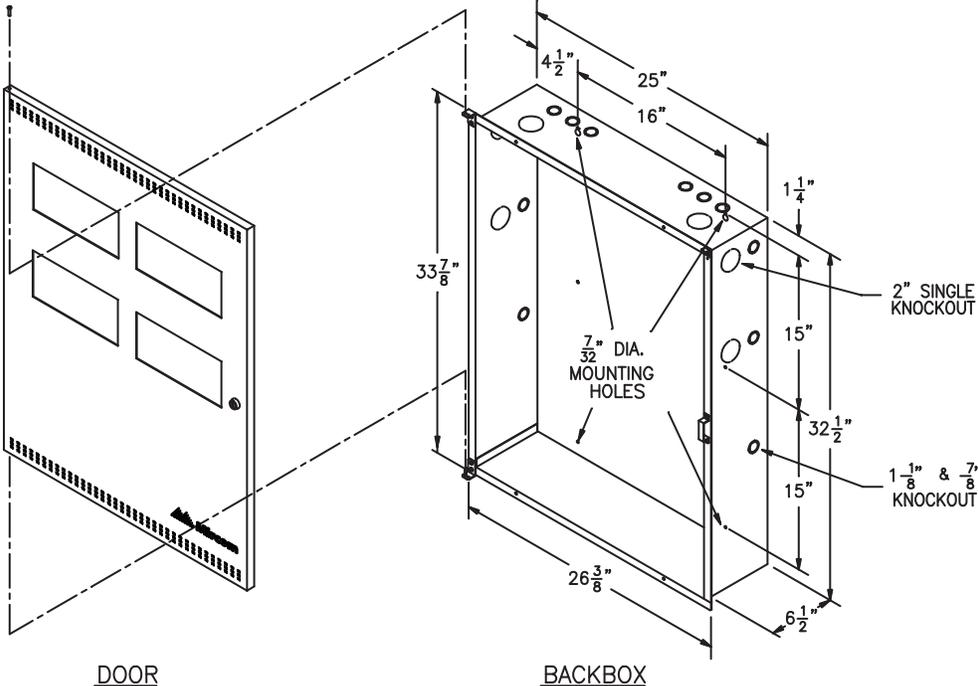
Figure 3: BB-5008 Enclosure Installation Instructions and Dimensions
