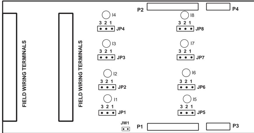
**P2:** Data cable to P6 or P5 of main fire alarm module, or to previous adder module.
