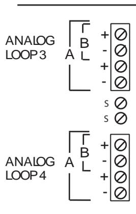
This board is mounted over the ALCN-792MISO to provide an additional two loops, for a total of four loops.
