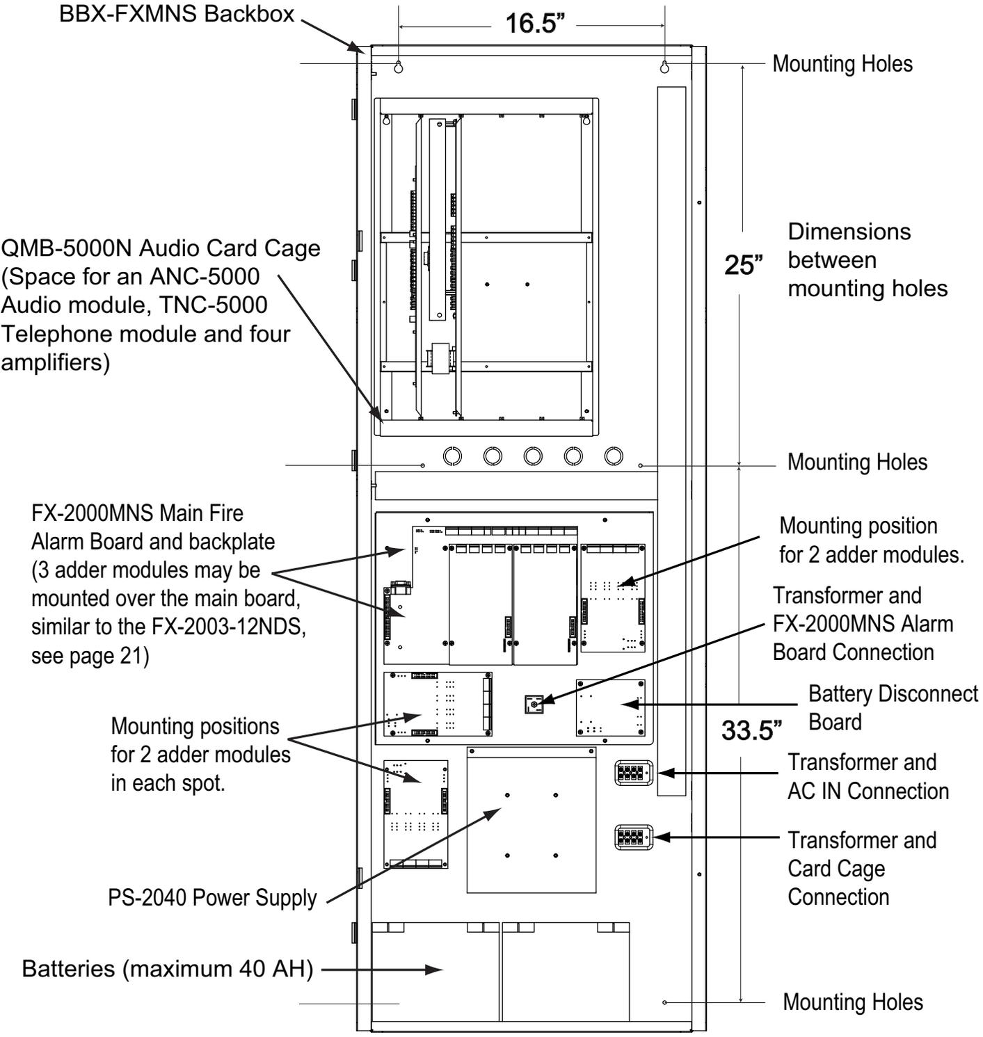
Figure 49: BBX-FXMNS Enclosure Complete View
