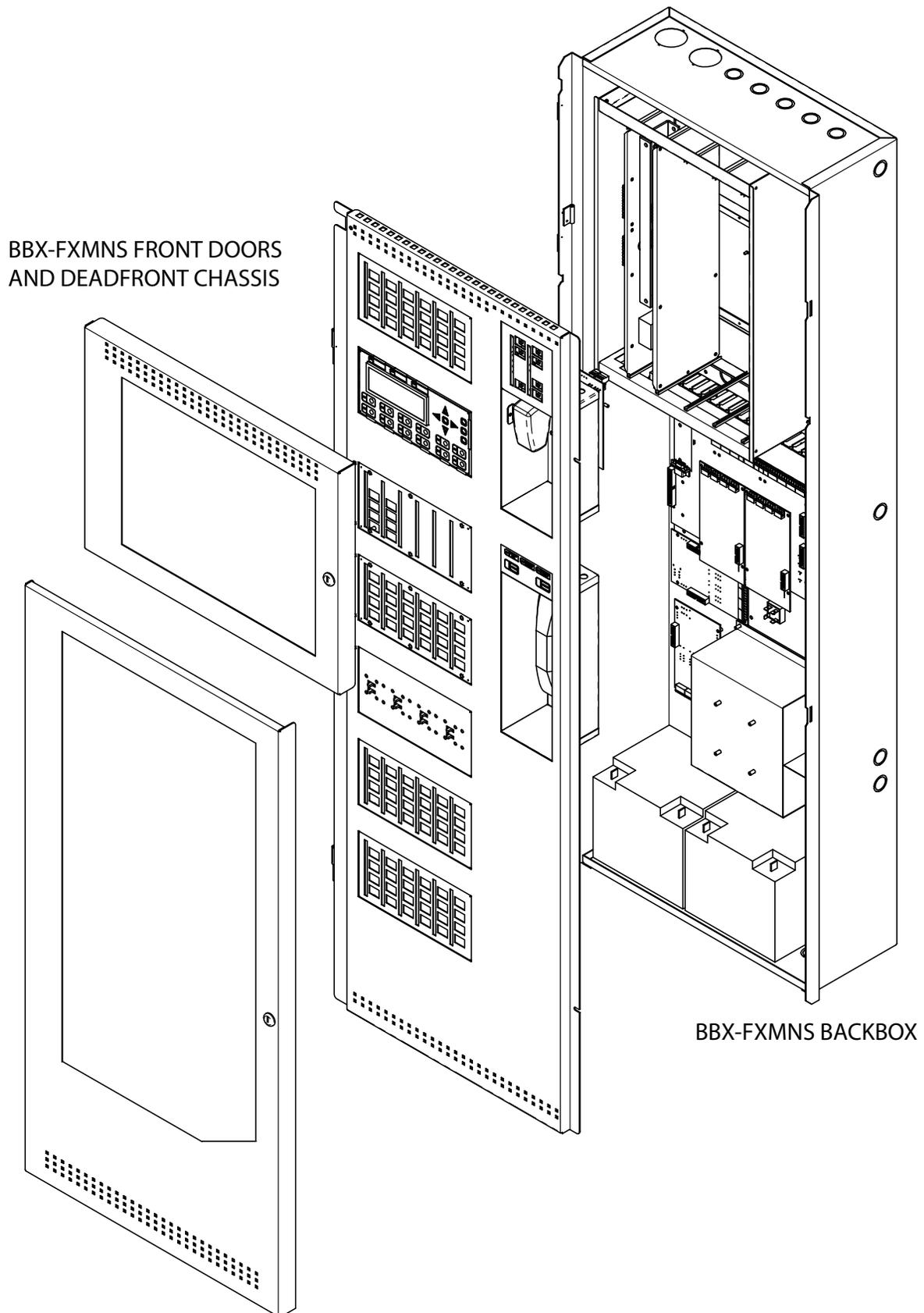
Figure 50: Mounting Vertical Microphone and Telephone Modules in the BBX-FXMNS
