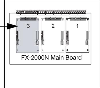
The recommended mounting position is 2 for the FNC-2000. The FOM-2000-UM board, if used, is mounted over the FNC-2000 board.
