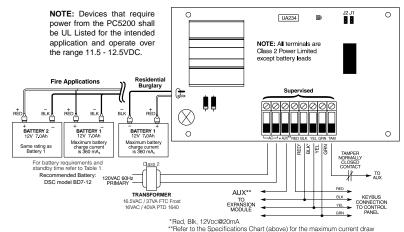
**AC** - Supervised, the PC5200 requires a 16.5V/37VA or 16V/40VA transformer. Connect primary of the transformer to an unswitched AC source (maximum current draw 0.5A) and connect the secondary of the transformer to these terminals.
