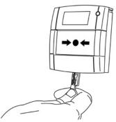
To test the Call Point simply insert the special test key (provided with every unit); the glass drops and the switch closes. Removing the key restores the Call Point to normal.
